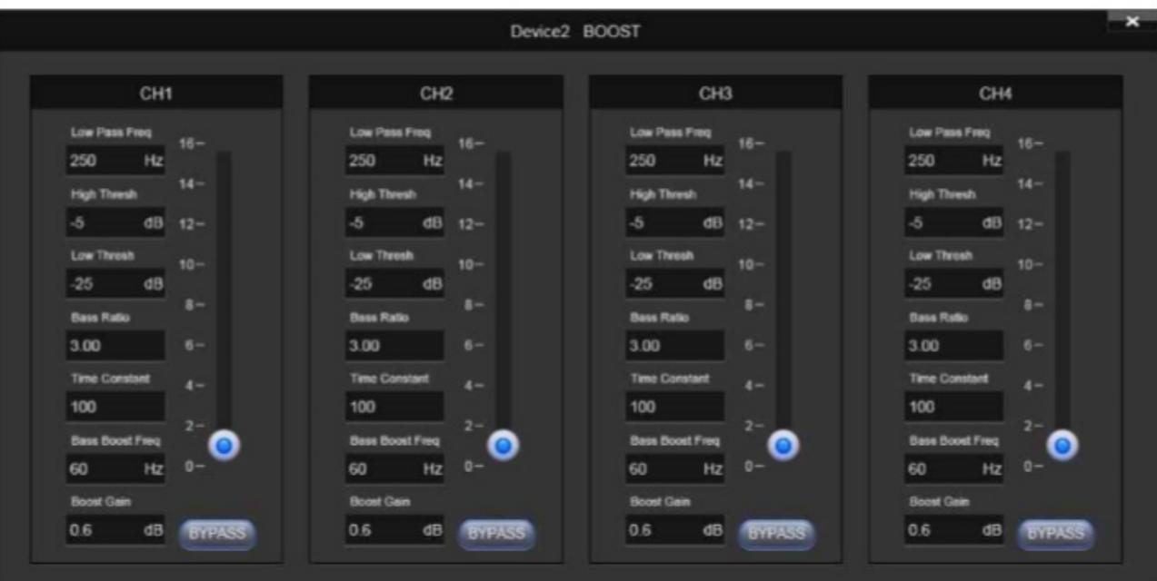
**Lowpass Freq:** The lowpass frequency ranges from 20Hz to 250Hz; frequencies below the selected point are used by the detector for determining the boost amount.
