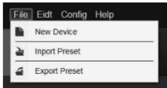
2. New device, you can select the device type, AK2-DSP or AK4DSP series, 700W and 1300W, select the device ID, modify the device name.
